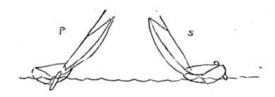
It is quite clear that the port tack vessel has its steering board "dug in" more deeply and will respond better than the starboard tack boat, which may have its steering board lifted almost clear of the water. Again the less maneuverable boat is given right of way over the more maneuverable one. Starboard has right of way over port.
